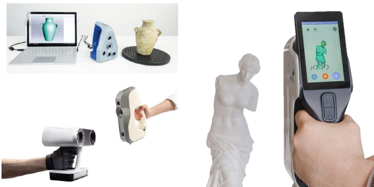
Figure 13. Light structured scanner by Artec 3D (on left); example of digitising of a statue (on right).
