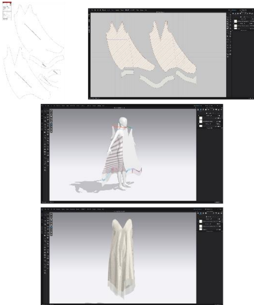
Figure 18. Example of creating a 3D asset from a digital pattern in CLO3D.
