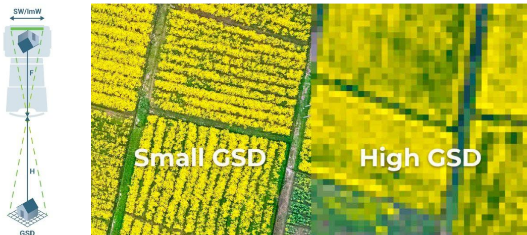
Figure 14. Example of choosing different values of GSD and the impact on final results.
