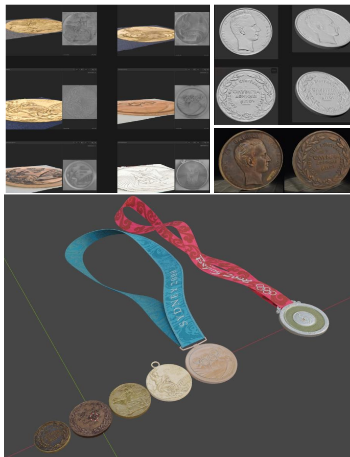
Figure 25. Process for creating 3D models of medals, starting from high-resolution images and the preliminary 3D model to the final objects.
