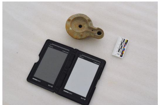
Figure 32. Colour correction, white balance and measure recording while digitising an oil lamp.
