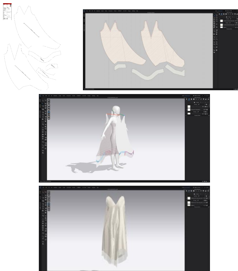
Figure 11. Test on the Digital Objects n. 1 (ST2202). Top left: digital pattern of the dress. Top right: pattern upload in CLO3D. Middle: creation of a 3D model. Bottom: 3D textured model 22 .
